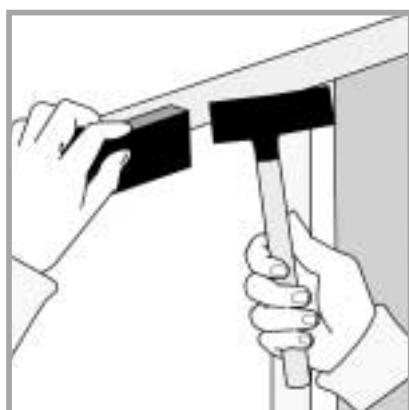
7 Tap the inner flanges to their place. Note: Always use a shock damper, for example, a piece of wood.
